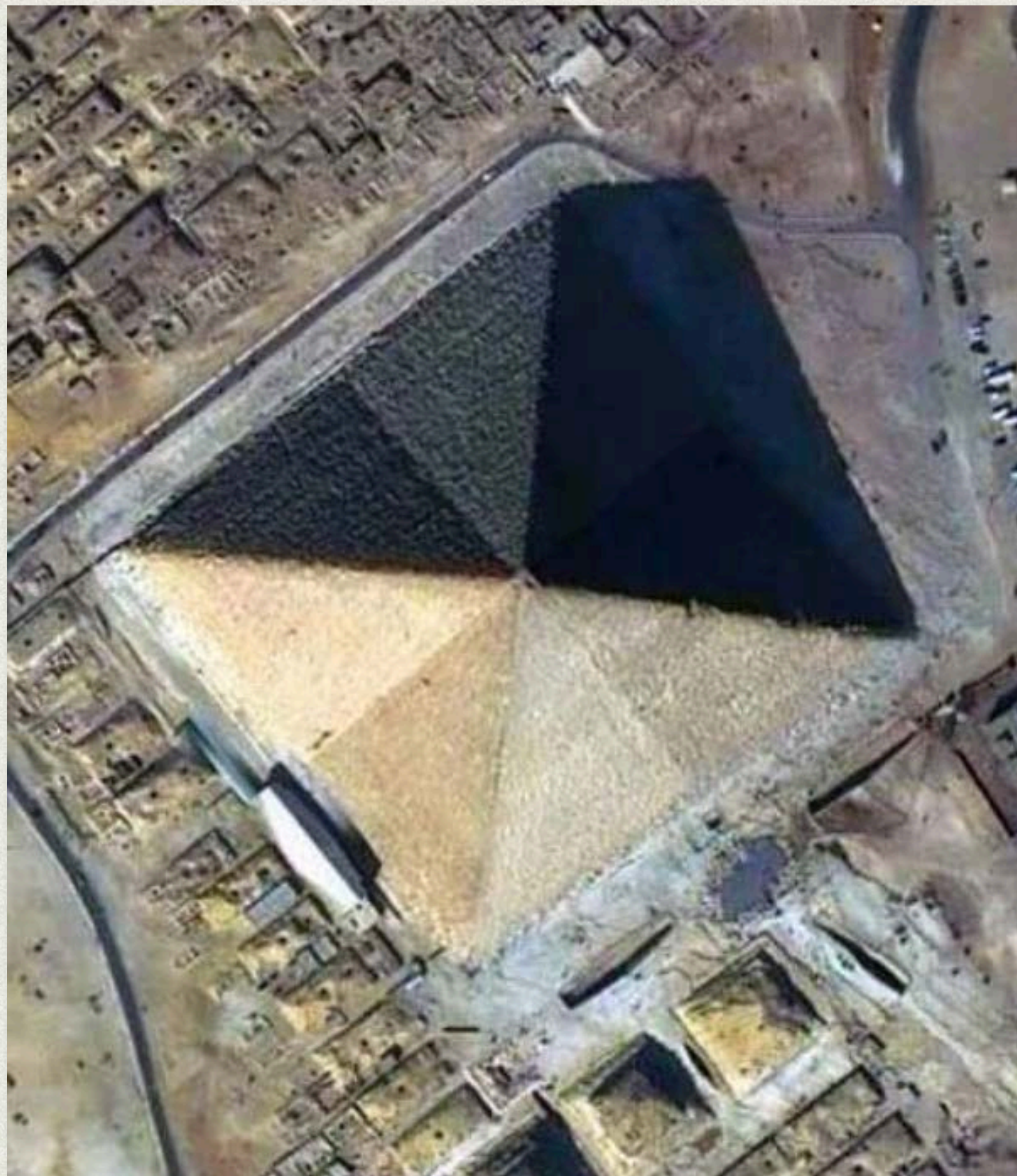
Aerial view of the of the Great Pyramid revealing the eight facets of its four sides
