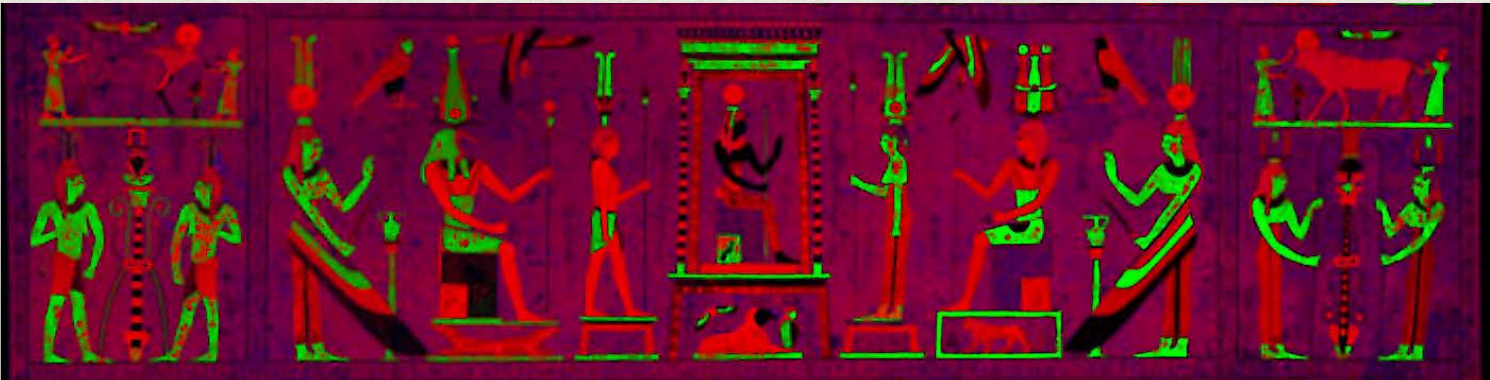
RGB false color overlay of MA-XRF distribution maps of copper (red channel)
